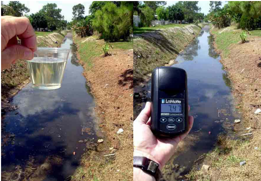
Clarity: The actual NTU value of the discharge water was read at about 7.5 NTU. The clarity and color of the water speaks for itself.
